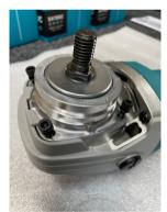
Step 02: Place four hex standoffs (spacers) over empty screw threads. Fit shroud on top, lining up holes with the standoffs. Next, fit washers and long screws, pulling the gearbox and shroud firmly but carefully together. Avoid over-tightening!
