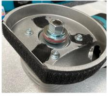
**Step 03:** Attach rubber hose by pressing it firmly onto the shroud outlet.
